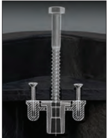
Non-Seizing Bolt System Allows Field Replacement
