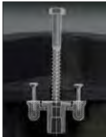
Non-Seizing Bolt System Allows Field Replacement
